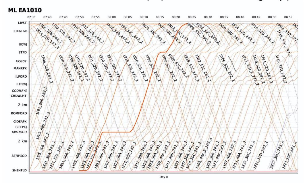
In this simulation a train alarm triggered an emergency stop lasting 8' between Harold Wood and Gidea Park with the subsequent trains gradually recovering the line delay.
