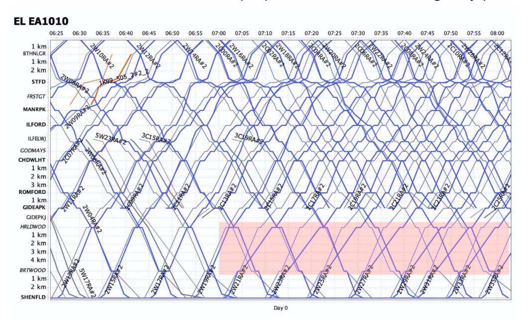
In this simulation the ATO failure at 7.00 a.m. starting at Brentwood for the next 5 km requires to lower the train speed to 36 km/h
